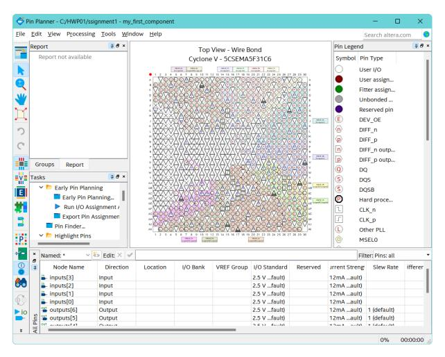
We see the BGA side of the FPGA chip that we've selected. Our goal is to connect our signals to one of the pins of the chip. We cannot just arbitrarily select some pins because our FPGA resides on a given circuit board. Luckily we have the schematics and a user manual for the board.
