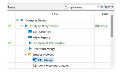
The RTL viewer will show the register transfer level schematic of your design.
