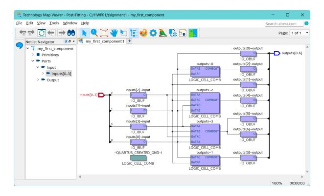
Here we see that it uses just a few logic elements. This is only a tiny fraction of the number of logic elements available (over thirty thousand).
