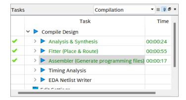
This step usually takes a relatively long time, compared to compiling a small piece of software, for example. This is another reason why we want to simulate our design before implementing it into the FPGA.
