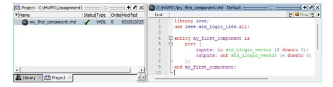
Note that the status of the component has also changed to a green  $\checkmark$ . This means it compiled successfully. If it didn't compile successfully it would show a red  $\checkmark$ . Even though we compiled the component, we cannot simulate it, because we have not declared how it should behave. This can be done by adding the **architecture** section to the code.
