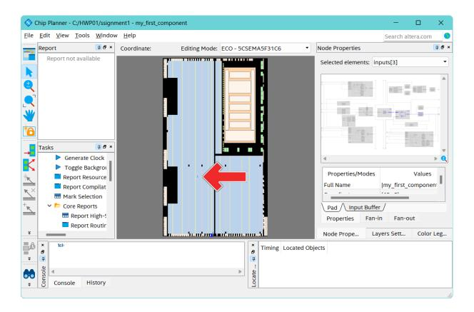
This is a schematic view of the FPGA chip itself, and it also shows which elements of the chips are used. Only one region is used, and most of the time the unused regions are shut down to save power. The bigger your design is, the more power it will therefore use.
