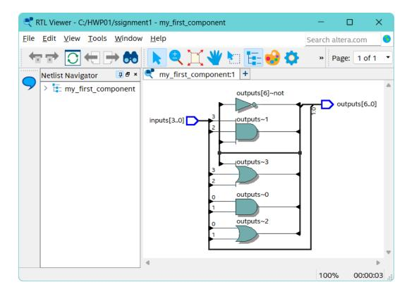
Here we may see the logic function that our architecture implements with the given inputs and outputs.
