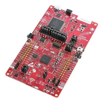
Figure 2.2: The CC3220 LAUNCHXL SimpleLink™ Wi-Fi® LaunchPad™ Development Kit.
