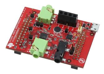
Figure 2.1: The CC3200AUDBOOST Audio BoosterPack.
