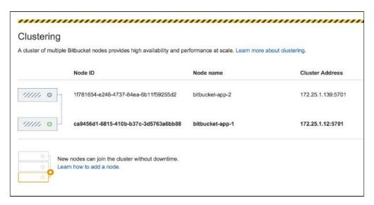
Verify that the new node you have started up has successfully joined the cluster. If it does not, check your network configuration and the  $\{BITBUCKET\_HOME\}/log/atlassian-bitbucket.log files on all nodes. If you are unable to find a reason for the node failing to join successfully, contact Atlassian Support .$
