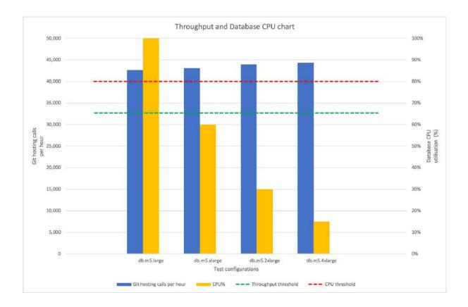
Only **m5.large** failed the CPU utilization threshold. All other tested virtual machine types are acceptable, although, **m5.xlarge** is pretty close to our CPU utilization threshold at 60%.
