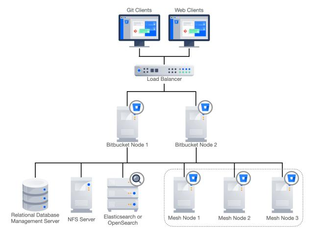
A minimum of three Mesh nodes must be deployed because this is the minimum supported replication factor required for the system to sustain a failure of one node and still form a write quorum. Any number of Mesh nodes three or greater can still be deployed, as this may be needed to scale processing, storage, or networking capacity.
