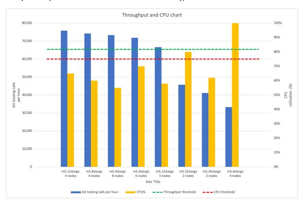
We have also carried out performance testing on 2 nodes (96 CPUs), but this resulted in poor performance, not meeting the threshold. Test results showed that 2 node deploys are not suitable for xlarge load. During the 2 node tests, the time spent on kernel was very high, which was not evident on 4+ nodes.
