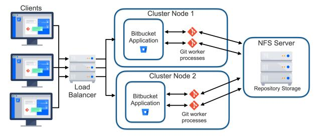
However, it can be challenging to build a truly highly available NFS server. The standard supported NFS deployment is a Linux-based NFS server. While this system may be built with redundant disks, power supplies, and network interfaces, it's still a single node and subject to failures. Besides, it can't be restarted for maintenance (such as operating system patching) without a Bitbucket system outage.
