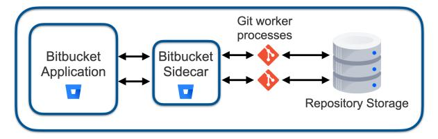
Generally, the sidecar is a concept that isn't important to the operations of your Bitbucket instance. Where previously the Bitbucket application made Java method calls to access process-local SCM code, now it makes a gRPC call to the sidecar process to do the same. The primary areas where the administrator needs to be aware of the existence of the sidecar are monitoring and troubleshooting.
