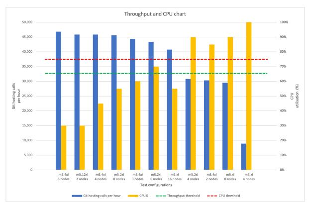
CPU is underutilized at 30% for the following application node configurations:
