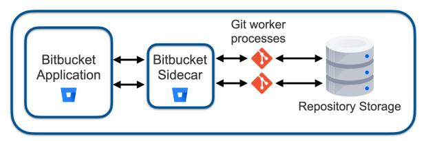
Where previously the Bitbucket application made Java method calls to access process-local SCM code, now it makes a gRPC call to the sidecar process to do the same.
