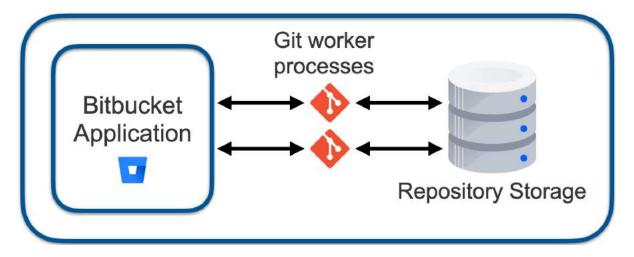
In a multinode Bitbucket cluster deployment, the repository storage is hosted on a remote NFS (see Figure 2). In such a system, I/O latency for similar operations is 10 to 1000 times slower due to the necessity of requests transiting the network, and due to the shared nature of the filesystem, many things can't be cached on the NFS client (that is the cluster node) but can only be cached on the NFS server, thus still incurring network latency overheads.
