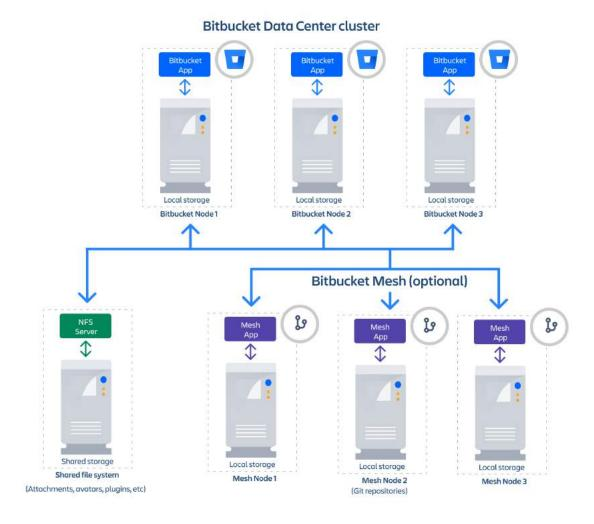
Bitbucket DC 8.x with 3 cluster nodes and 3 Mesh nodes
