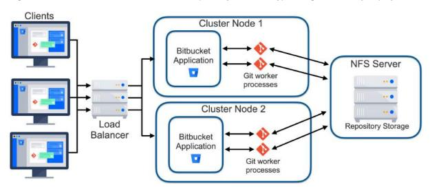
However, it can be challenging to build a truly highly available NFS server. The standard supported NFS deployment is a Linux-based NFS server. While this system may be built with redundant disks, power supplies, and network interfaces, it's still a single node and subject to failures. Besides, it can't be restarted for maintenance (such as operating system patching) without a Bitbucket system outage.
