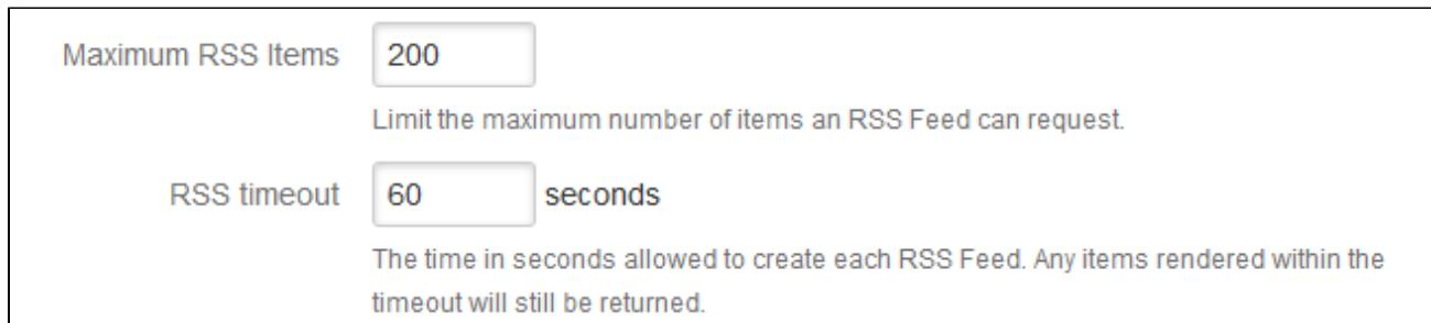
The screenshot shows a configuration interface for RSS feeds. It has two main input fields: 'Maximum RSS Items' set to 200, and 'RSS timeout' set to 60 seconds. Below each field is a descriptive text explaining its purpose.
