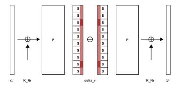
The algebraic computation is essentially equivalent to solving a related cipher of  $2(N_r - r)$  rounds (from C' to C'' via the predicted difference  $\delta_r$ ) with a symmetric key schedule, using an algebraic meet-in-the-middle attack.
