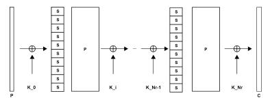
Where S is the 4-bit S-Box and P a permutation of bit positions.
