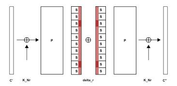
The algebraic computation is essentially equivalent to solving a related cipher of  $2(N_r - r)$  rounds (from C' to C'' via the predicted difference  $\delta_r$ ) with a symmetric key schedule, using an algebraic meet-in-the-middle attack.
