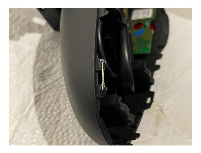
Allow the Araldite 16 hours to harden. Once hardened the clips are functional.
