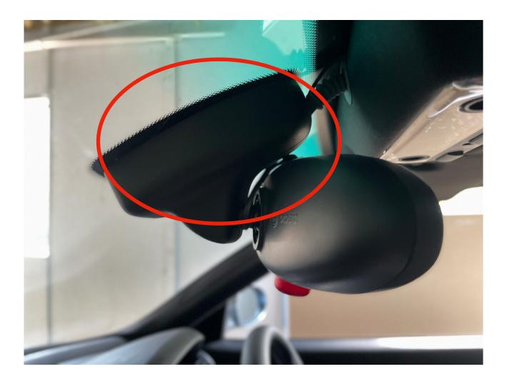
In order to remove the trim covers, insert the tip of the small trim removal tool (Tool A) into the join where the two trim covers meet.
