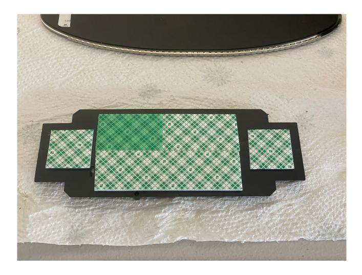
Seat the PCB back into the mounting bracket.
