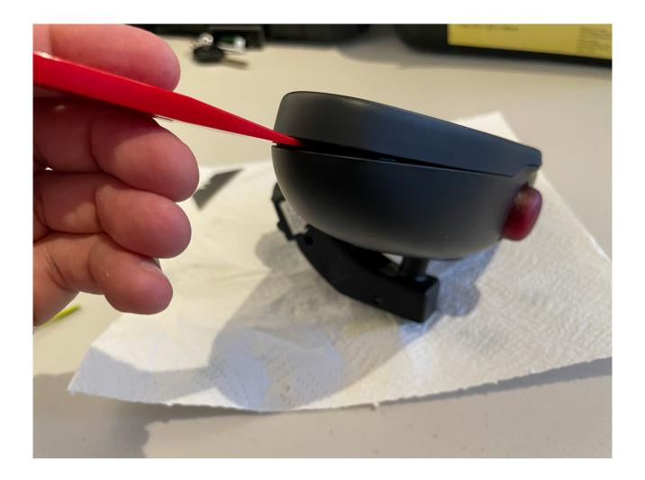
Carefully work around the mirror lifting the front trim piece so that the clips separate (refer to reference image on page 9 if needed).
