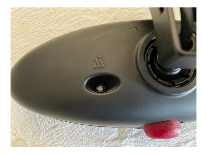
Next seat the new electrochromic mirror glass into the front mirror housing bezel. Ensure that the mirror is oriented correctly. The + terminal is at the top and the - terminal is at the bottom (which also has the hole in the bezel for the rear facing light dependent resistor).
