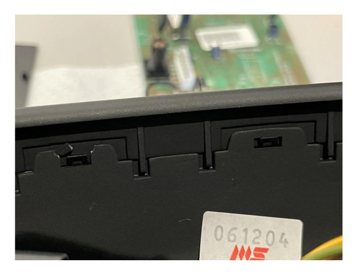
These clips are extremely delicate, especially on original mirrors which are now nearly 20 years old. Even being extremely careful it is almost impossible to avoid breaking at least some of the clips (as can be seen in the photo).
