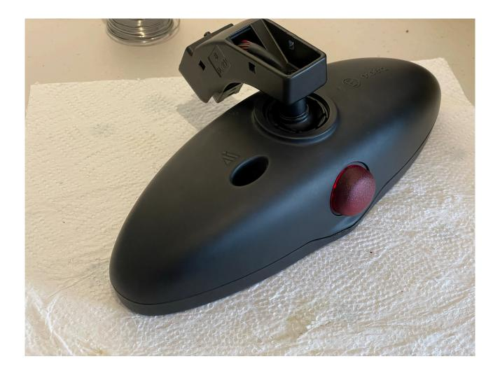
If the bezel is not held firmly and tightly in place then too many of the clips have been broken. It is recommended that you follow the instructions in Section 7 to repair the broken clips.
