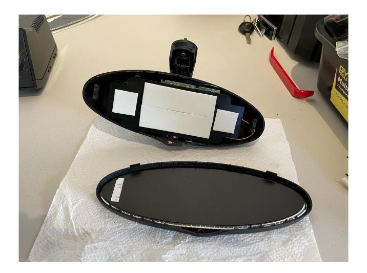
Remove the backing from the adhesive tape, then holding the mirror housing, use one finger on each side to hold the PCB mounting bracket in place. Rotate the mirror housing so that the adhesive tape is facing down. Gently mate the mirror housing with the front bezel, ensuring that the two are aligned. Do not actually clip the mirror housing to the front bezel.
