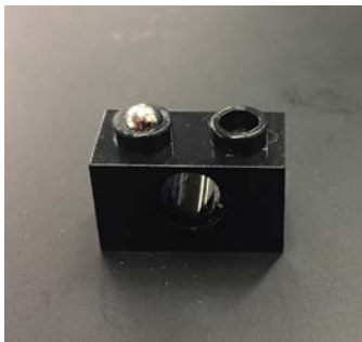
Figure 1. 1x2 Lego brick with 1/8” steel bead inserted into top cylinder.
